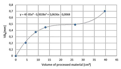
**Fig. 7.** Diagram of the dependence of cutting edge wear  $(V_{BB})$  on the volume of machined material for high feed milling with CS300 insert for machining parameters:  $v_c = 800 \text{ m/min}, f_z = 0.5 \text{ mm/edge}, a_e = 70.54 \text{ mm}, a_p = 0.5 \text{ mm}$
