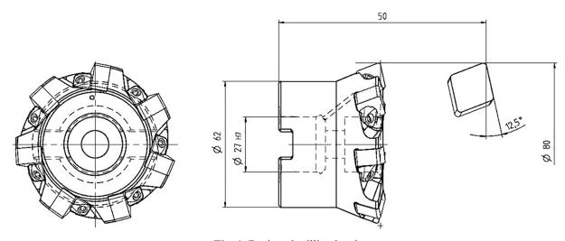
Fig. 1. Designed milling head
