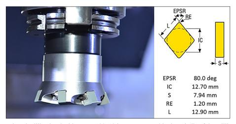
Fig. 3. Designed milling head with CNGN120712 inserts, mounted in the spindle of the milling center
