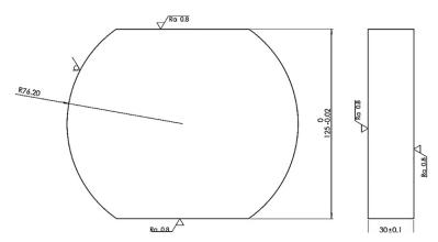
Fig. 2. A sample for testing made of Inconel 718
