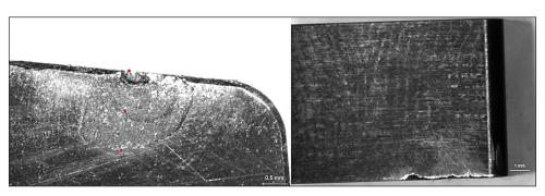
**Fig. 5.** Microscope image of the flank face of the CS300 insert for high feed milling (optical magnification 0.5x). Microscope image of the rake face of the CS300 insert for high feed milling (optical magnification 1.6x)
